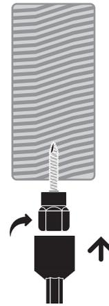
Attach the Hangerz® to the correct size socket driver and install anchor perpendicular to the base material substrate. To avoid over tightening it is recommended you use the HZSM10D Driver.
