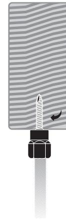
Install the threaded rod. The threaded rod should be fully installed into the Hangerz® anchor.
