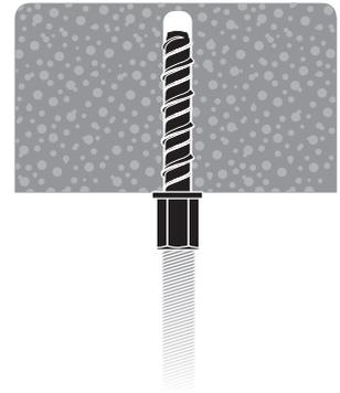
The head of the anchor should be set flush with the base material. Install the threaded rod.
